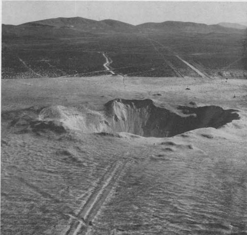
CRATER dug by Scooter blast measured approximately 300 ft. in diameter. It was 80 ft. deep at its deepest point. The test yielded information on cratering effects.
